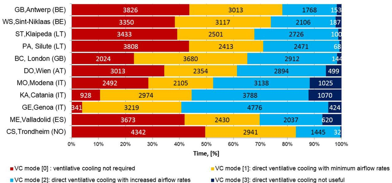
**Figure 2.** Percentage of hours within a year when direct ventilative cooling is required, useful or not useful in the eleven reference case climates when the specific lighting power is 30 W/m<sup>2</sup>.
