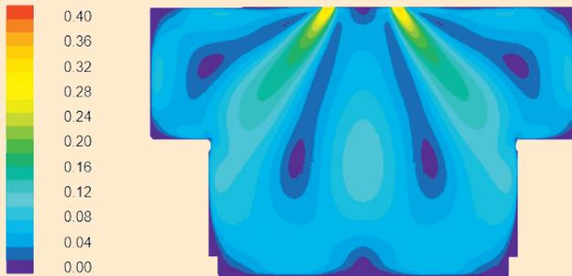
*Air velocity contours in the aisle between two opposite vertical display cabinets*
